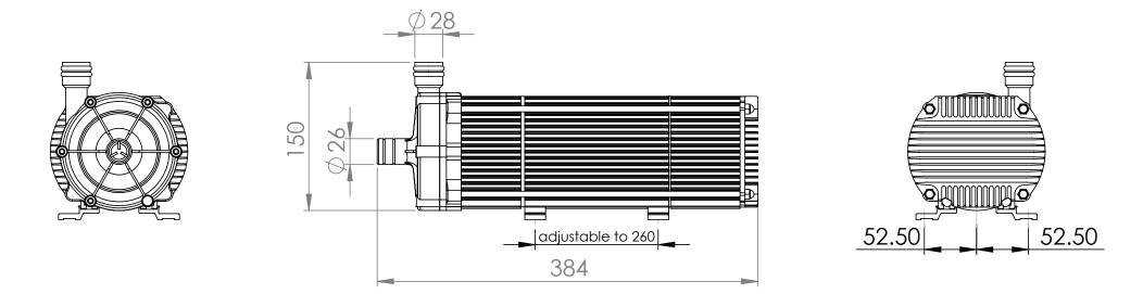
Inlet/Outlet front casing subject to change in order to suit customer requirements. Outlets on all JEC Marine pumps are rotatable in 60° steps.
